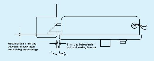
Although the lock is designed to suit most common applications, adjustment of loading spring tension might be required depending on the type of shutter and closing force. If the shutter is not getting locked, then loosen the tension by turning the hexagon nut (using 12 No. wrench). If the shutter is getting closed loosely, then increase the tension by turning the hexagon nut to make it work perfectly.
